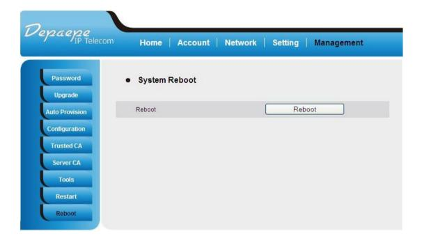
You can reboot the HD2000IP by clicking on the "Reboot" button after each update to the configuration page. Alternatively, you can reboot by unplugging the power supply of the HD2000IP and then powering it on again. If your HD2000IP ever becomes "stuck" or un-responsive, you can unplug the power supply to reboot it. Frequent rebooting by unplugging the power supply is not recommended and should not be necessary.
